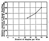
Fig. 51.—Tests of wire-bound boxes for two dozen No. 3 cans; relation of number of staples to amount of rough handling required to cause loss of contents.
